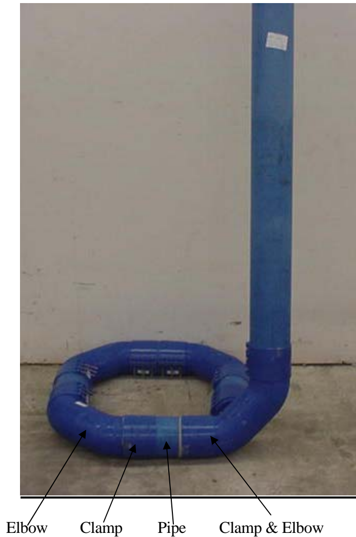
View of the test mockup
